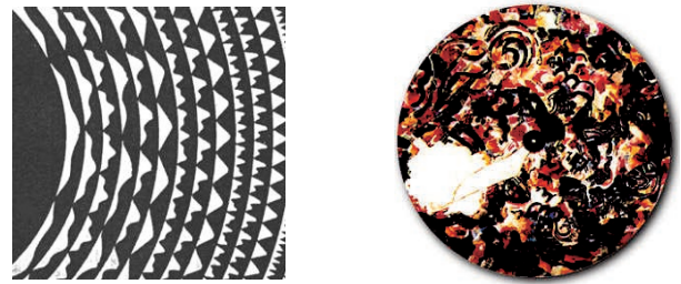
Figure 2: Examples of disks used by Welte Light-Tone (left) and Piano Optophonique (right)
