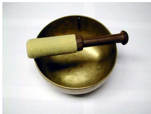
Figure 2: The HyperPuja stick with a Tibetan singing bowl. The magnet for the hall effect sensors can be seen inside the bowl.
