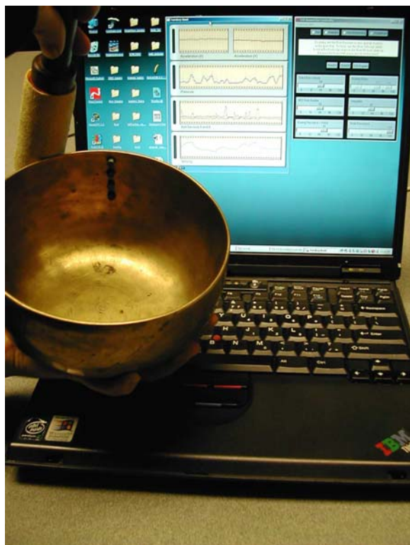
Figure 3: The HyperPuja stick in performance. The laptop screen shows the sensor data display on the left and the sound synthesis GUI on the right.
