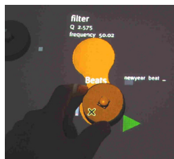
Figure 9c. As the user moves the puck, the settings change, and the highlighted area stretches between the puck's initial position and the new position.
