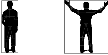
Figure 2. Silhouettes and their bounding boxes. The leftmost one has high contraction index while the other has low contraction index.
