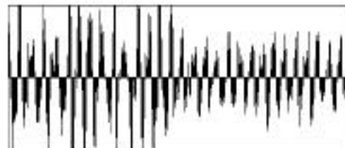
Figure 3. DC offset removal of pixel difference variation of video caption of a waving hand.
