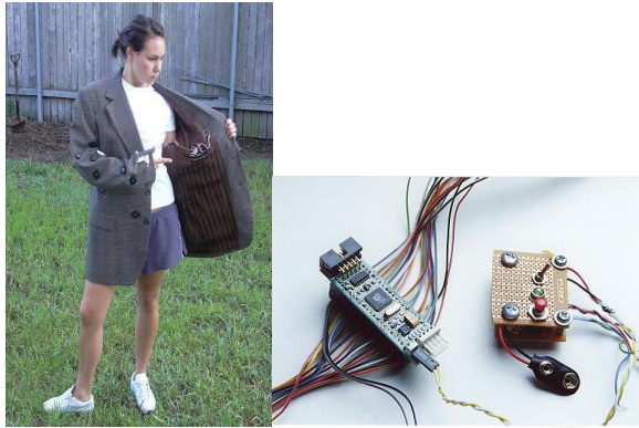
Figure 1. The Singing Jacket (2003) a sound installation designed, built and tested by Mark Havryliv. Sensors located at movable parts in the jacket allow the wearer to affect the sound algorithm.
