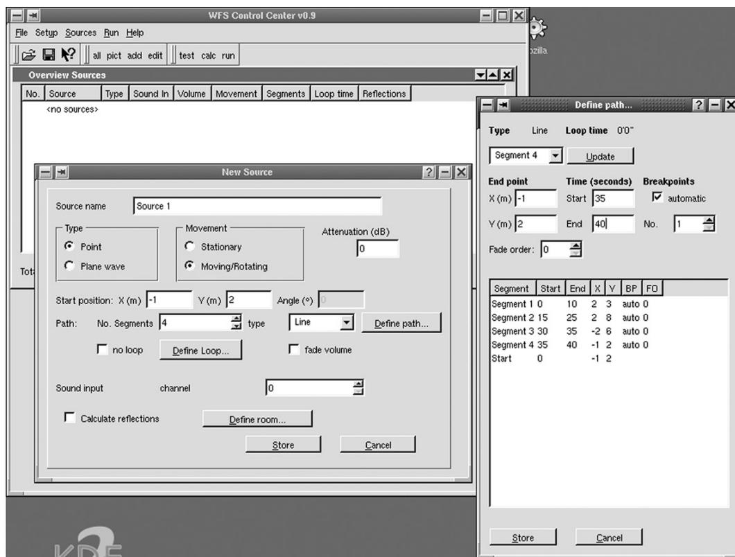
Figure 3. Screenshot of source and path definition. Graphical results of this input is shown in figure 4.
