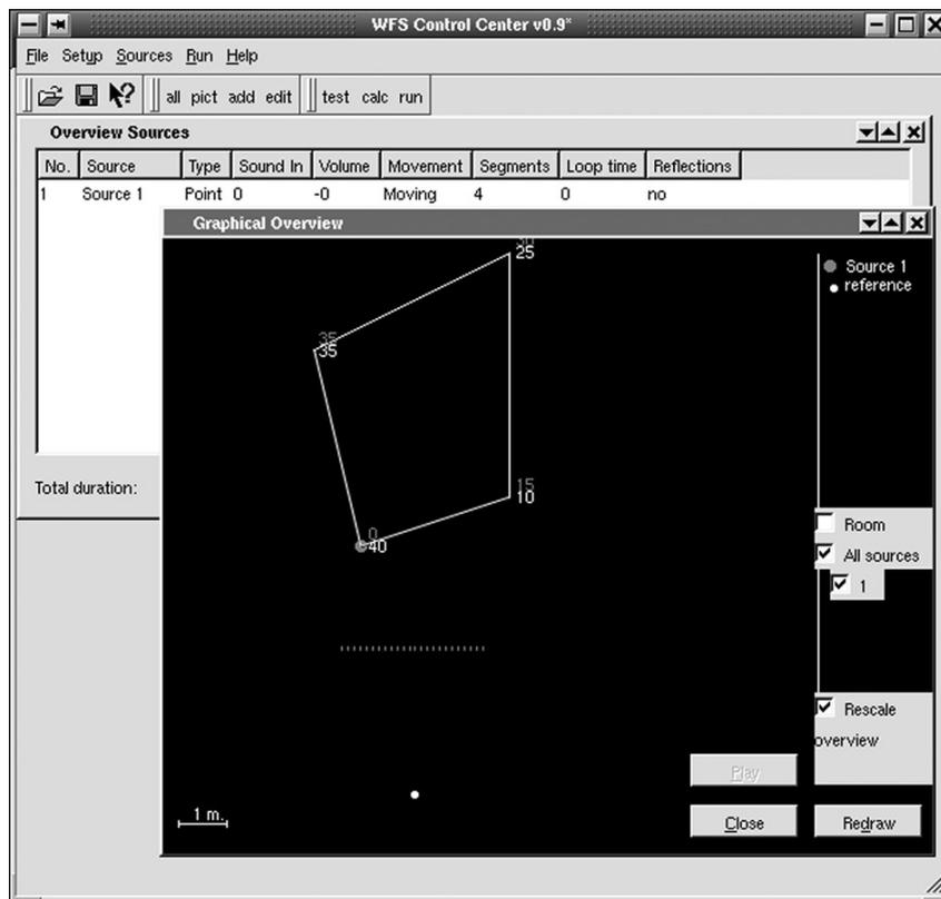
Figure 4. Screenshot of the graphical overview of the source path. The numbers at the points between segments indicate the departure (dark) and arrival (light) times. The dots in between the path and the reference point are indicating the loudspeaker array.
