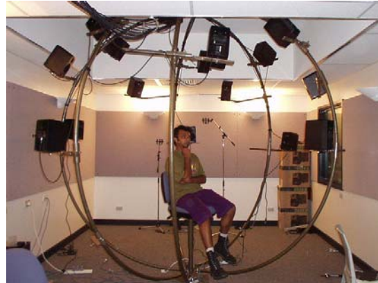
Figure 1: The CHES 16-speaker dome
