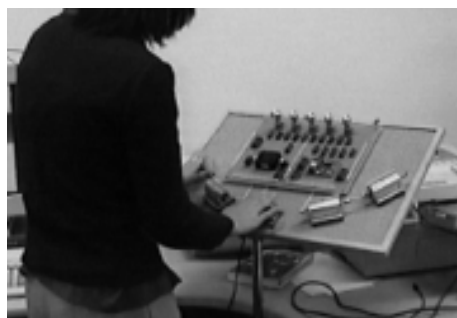
Figure 8. touch sensor for Improvisation-III
