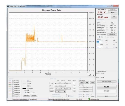
You can see the chip launch at about 1.5 seconds, then turn on the WiFi and at about 2s make the SSID connection and MQTT connection. The average current is about 100ms afterwards, and a packet spikes up to  $^{\sim}130$ mA at the 7 second mark.
