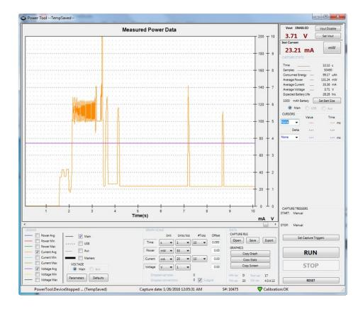
Note that 10mA or so is for the ATSAMD chip, so that means you've got ~12mA for the WiFi module.
