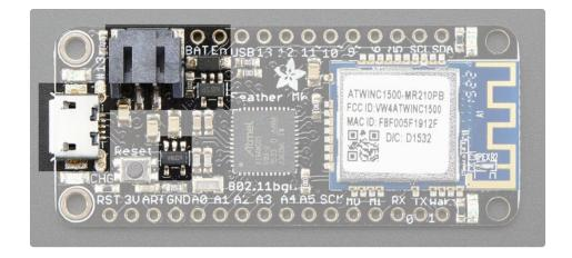
The above shows the Micro USB jack (left), Lipoly JST jack (top left), as well as the 3.3V regulator and changeover diode (just to the right of the JST jack) and the Lipoly charging circuitry (to the right of the Reset button). There's also a **CHG** LED, which will light up while the battery is charging. This LED might also flicker if the battery is not connected.
