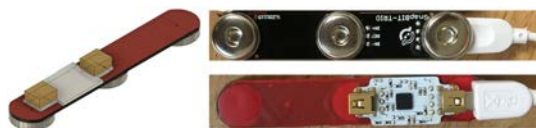
Figure 2: Plux's Snap Bit Trio with soldered EMG module.
