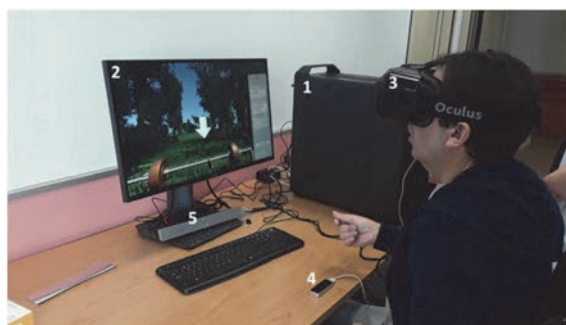
Figure 4. VR system used at the rehabilitation center. 1) Computer. 2) Monitor. 3) Oculus Rift head mounted display. 4) Leap Motion controller. 5) Speaker.
