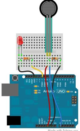
Connect USB and upload your code. Now you can control the brightness of your LED by pressing on the force sensor.
