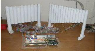
Figure 1. Light Pipes MIDI Controller
