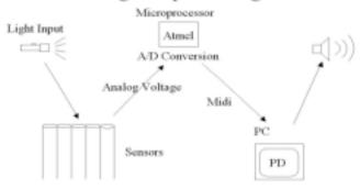
Figure 2. Light Pipes Signal Flow
