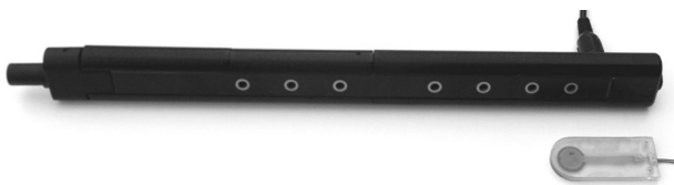
Figure 1: The Epipe showing the front 7 toneholes and the "Energy Input" FSR
