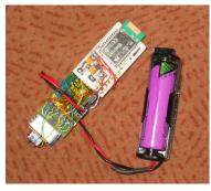
Figure 2. Aobachi embedded hardware powered by a AA size battery.
